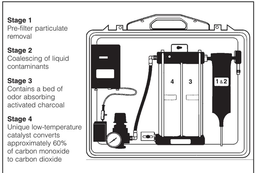
**3M™ Portable Compressed Air Filter and Regulator Panel, 256-02-00 (four-stage filtration)**
